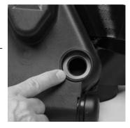
**Note:** When replacing the gasket(s), take proper care to ensure that the cartridge inlet port threads are not damaged.
