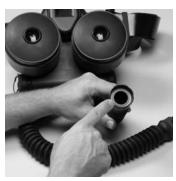
3. Attach the breathing tube inlet to the blower outlet connection and snugly hand-tighten.
